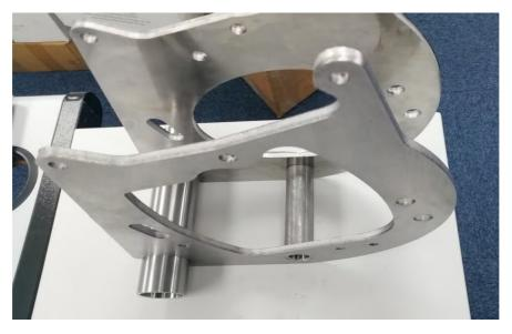
"Why bother?" I hear you ask, since 6mm plate is not that far away from ¼" (6.3mm). The problem is that the swinging arm mounting must be the correct width. 6mm plates will give you 0.6mm of immediate side play in the swinging arm mounting area where you can least tolerate it. Add to it other components like the crankcase and gearbox also need to fit to the subframe, so you cannot simply
