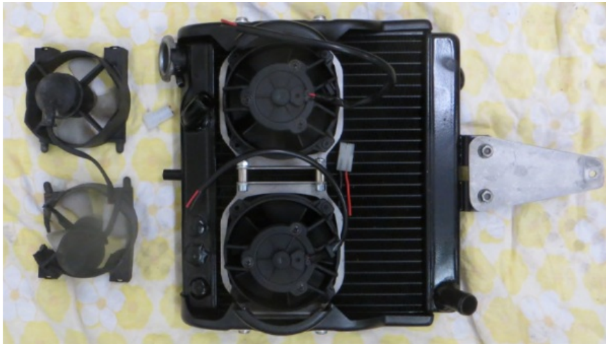
Original fans on the left, new fans on the radiator. Still missing correct electric connectors.
