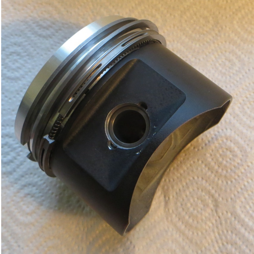
Above: coated piston, a trick Joerg Winkelmann has used on race engines with good results.
