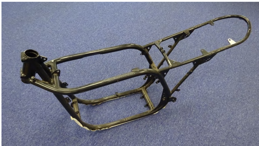
Above: the original factory lowboy frame Mick won races with in Japan with a Commando engine driving it. Originally fitted with an outside flywheel 350 works Manx engine as the flattened right hand tube reveals. Now all we need to rebuild it is a 350 outside flywheel
