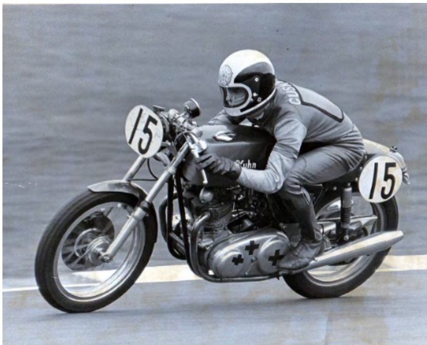
Dave Potter on a Gus Kuhn Commando. Same modification for the rear suspension mounting, but a brace between the front downtubes ours does not have. Picture from the Mick Hemmings files we bought last month.
