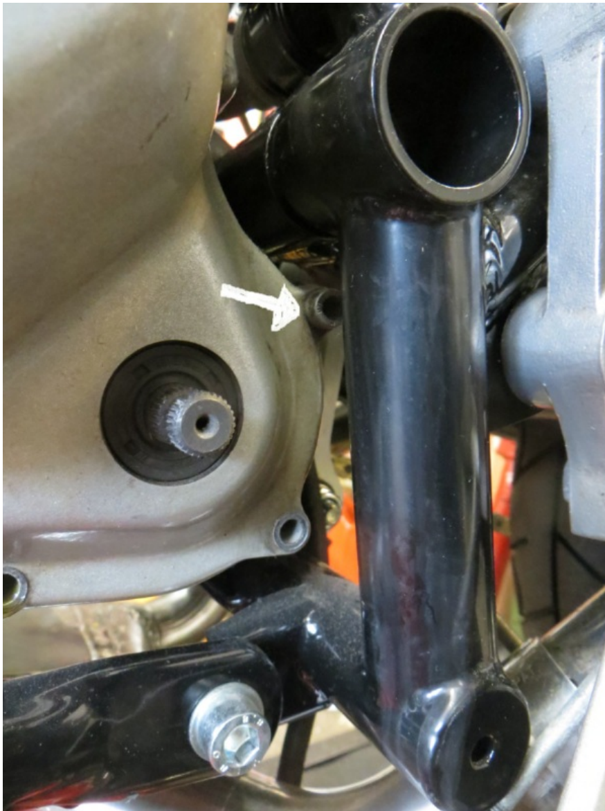
No way could I get at that allen screw. Even if, it was too long to be taken out.
