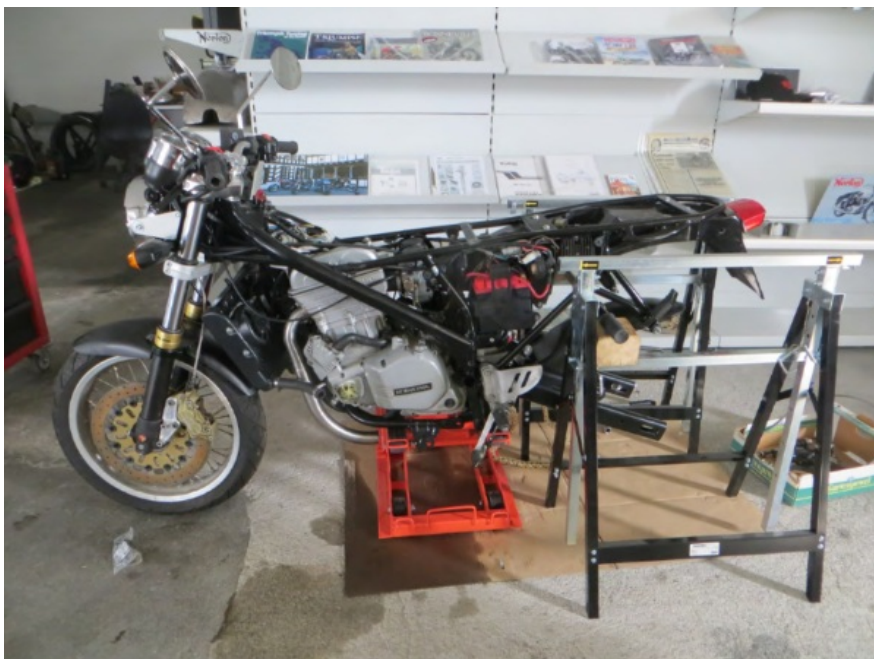
Enterprising system to suspend main frame and to maneuver the subframe with the engine!
