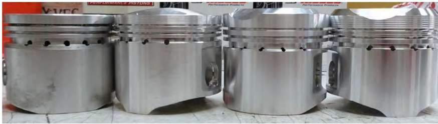
From left to right: GPM standard 750, Wiseco standard piston, Omega (forged) and the Wiseco AMA type piston.
