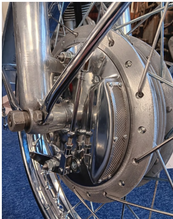
Above: New hub and new TLS brake plate test-installed.
