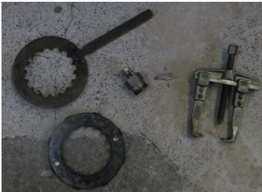
Above: Tools to take the primary off. The two on the right are leftovers
