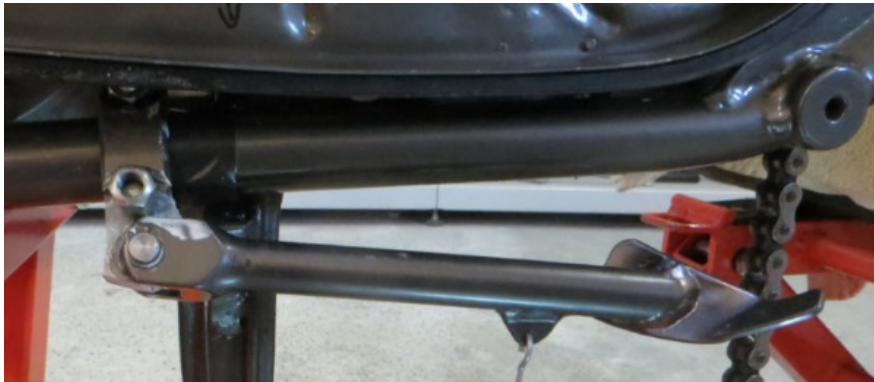
Side stand in situ. Tape with rubber buffer behind it since this was the first-ever featherbed production bike and no reinforcements had yet been found necessary to take the impact of the centre stand stops.
